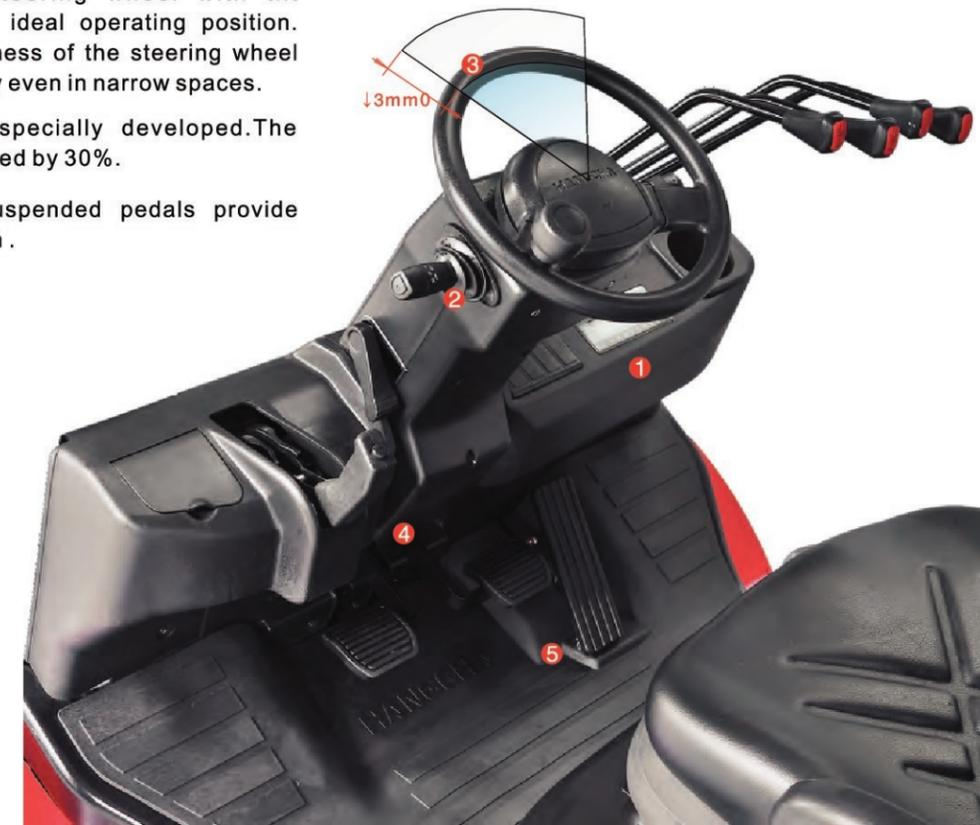
The new vehicle controller integrates all electrical components, features excellent durability for temperature, water and vibration for most demanding operation.
